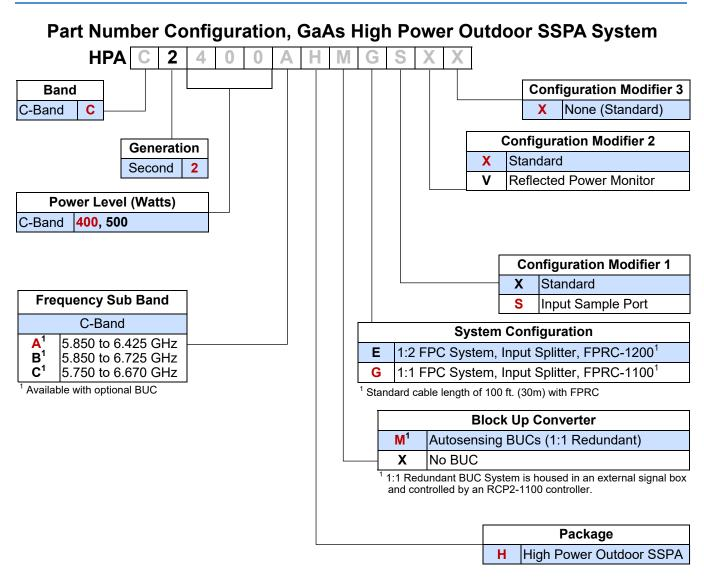
**Example** - A 1:1 Fixed Phase Combined 400W system utilizing two (2) GaAs C-Band High Power Outdoor SSPA with optional input sample ports and optional internal reference block up converters is part number: **HPAC2400AHMGSXX**.
