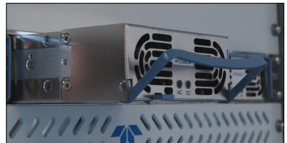
Power Supply Module in Chassis
