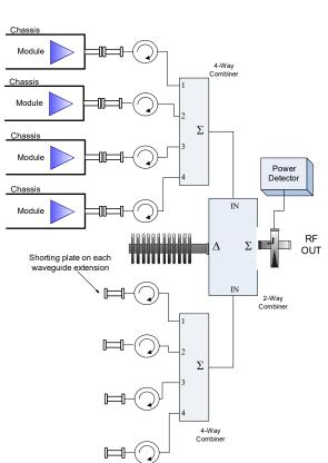
number of active modules vary. The Outdoor PowerMAX system is designed with an Auto-Gain Control mode so that the overall system gain will remain constant in the event of a single module failure. See the table below.
