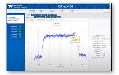
**Spectral view:** The Rx Spectrum Monitor is a powerful real-time spectrum analyser within the modem that is used to view the received signal spectrum. The monitor can not only display the wanted carrier but a Super Wide view allows checking for adjacent interfering carriers.
